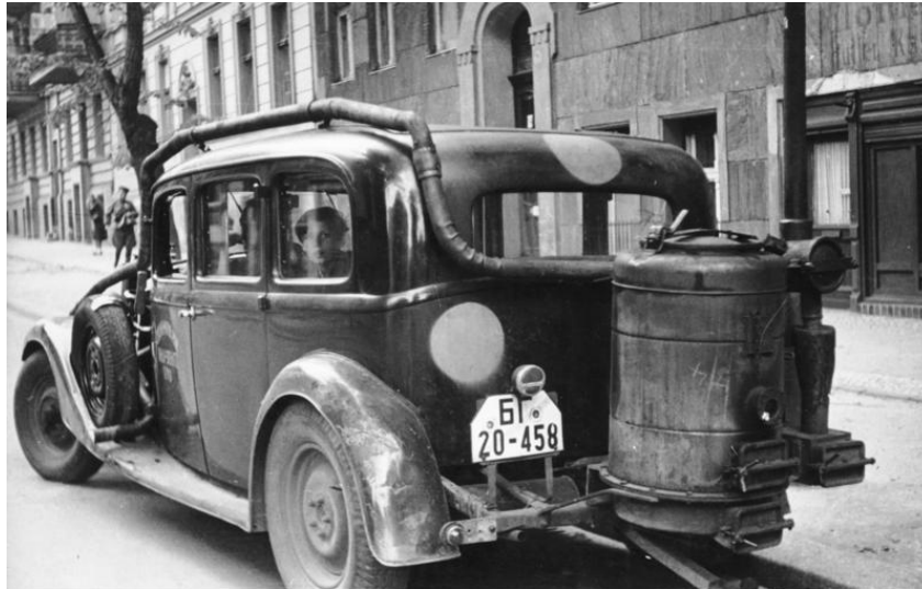
Figure 4: Car in Berlin 1946. See the “boiler” and the pipe that funnels the extracted wood gas into the internal combustion engine.
